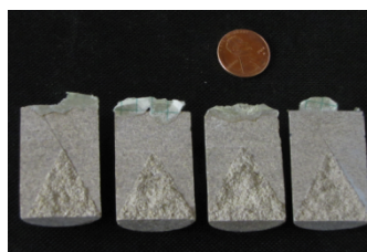
fractured short-rod specimens
