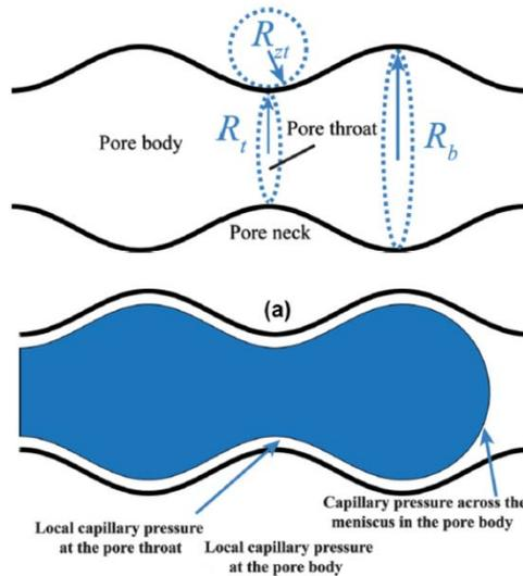
Capillary pressure or  $p_c$ :  $\Delta p = \left( \frac{1}{R_1} + \frac{1}{R_2} \right)$ ,  $R$ 's are principal radii of curvature
