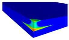
Distribution of CO<sub>2</sub> saturation for a maximum injection rate of 2.85 Mt/yr into a 30 mD injection zone and for the jointed representation of the caprock. Figure on the left is at 5 years, the end of the injection ramp-up period, and figure on the right is at 20 years.
