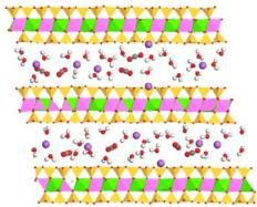
Intercalation of CO<sub>2</sub> and H<sub>2</sub>O molecules in in a montmorillonite clay interlayer. Color designation: red balls – oxygens; purple – sodium ions; white – hydrogens; gray – carbon.
